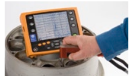
Rotary inspection of aircraft wheel tie bolt holes.
